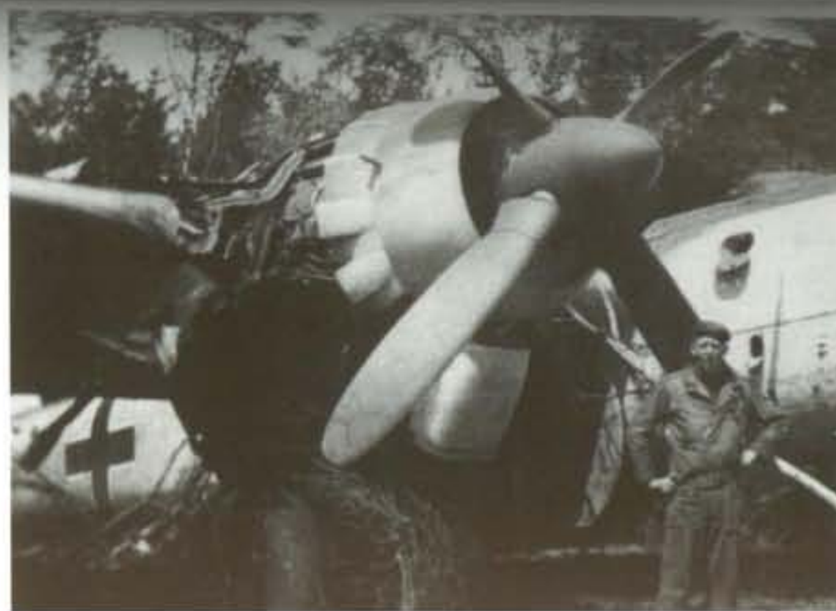
ABOVE: An Arado-built He 177 A-5 W.Nr. 550316 is seen here in an abandoned state after being found by US troops. Note how the last three digits of the Werknummer '316' are repeated on the tail fin and forward ventral gondola. The Heinkel also carries FuG 200 Hohentwiel ship search radar.
