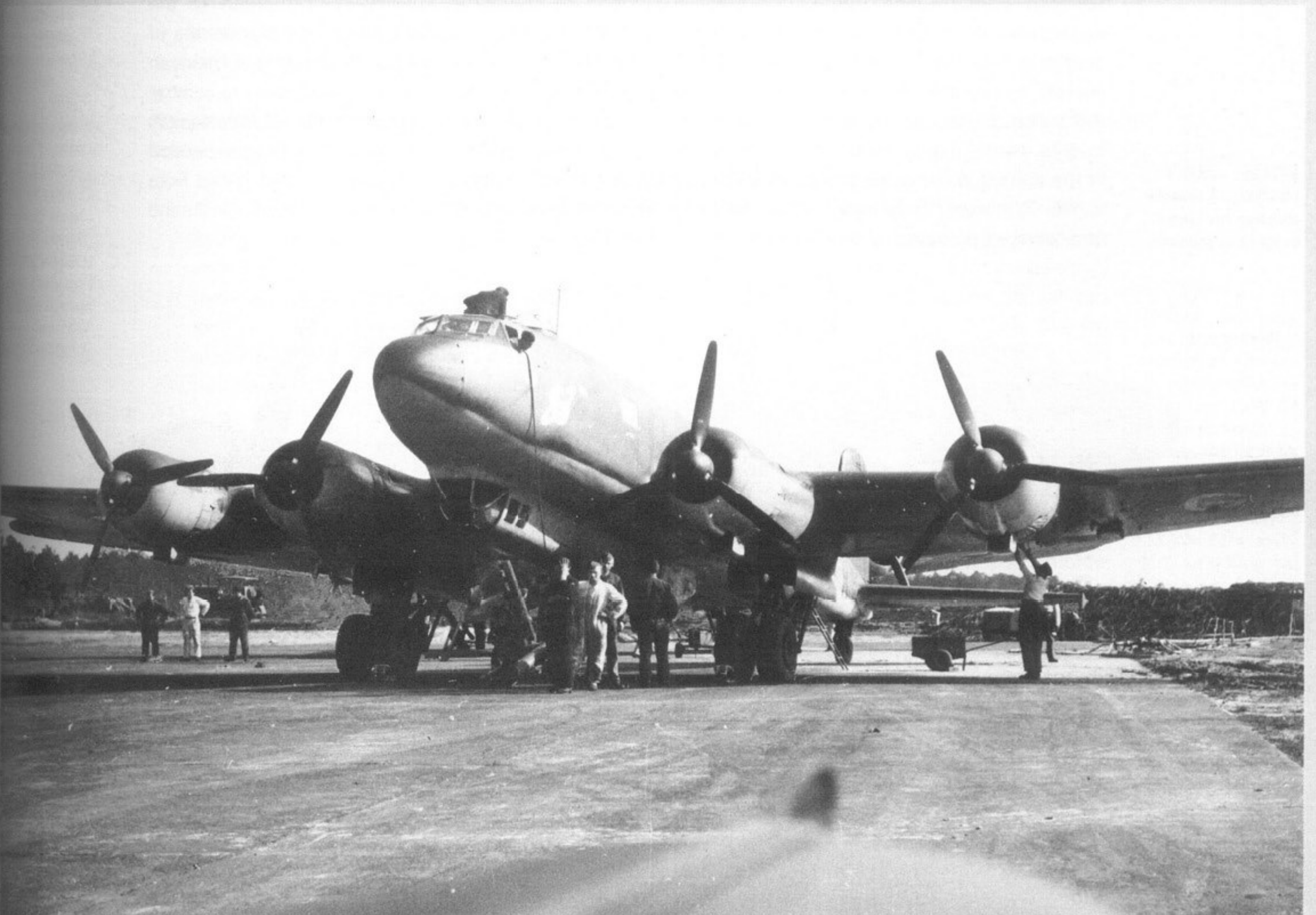
ABOVE: An Fw 200 C-3 of KG 40 undergoing maintenance on the ramp. The C-3 embodied major strengthening to the main spar and fuselage in an attempt to curb the structural failures. This model also saw the introduction of the low drag Fw 19 hydraulically-operated forward dorsal turret with a single 7.9 mm machine gun.
