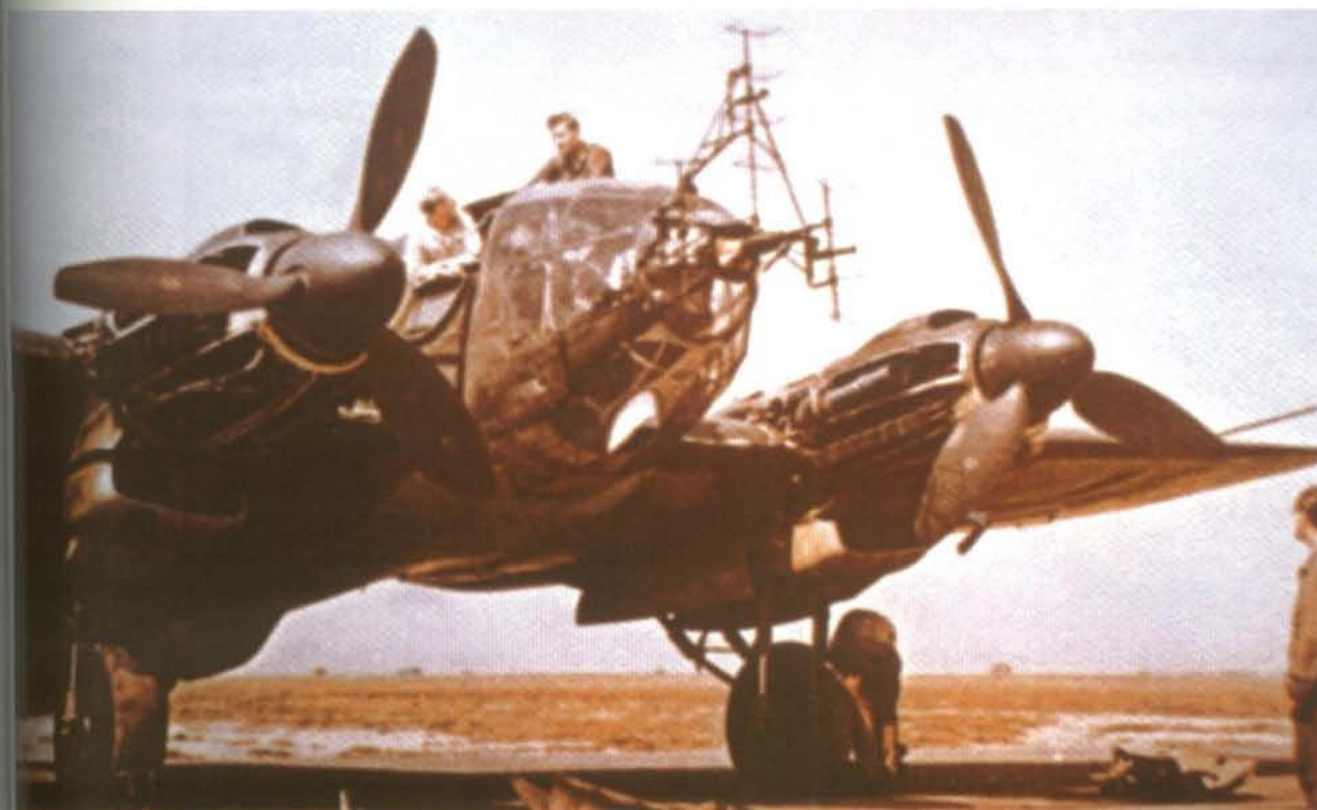
LEFT: A Heinkel He 111 of KG 26 fitted with FuG 200 Hohentwiel ship search radar.
