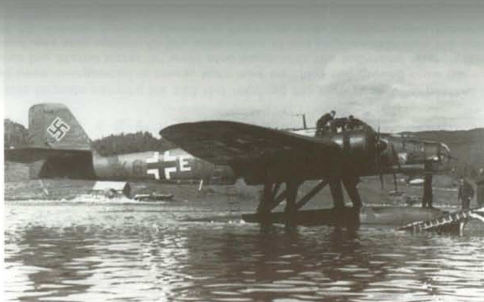
LEFT: Maintenance crews working on a He 115 C belonging to 1./Kü.Fl.Gr 406 coded K6+EH. In order to provide more defensive armament, this variant was fitted with an additional fixed MG 151 20 mm cannon under the nose.
