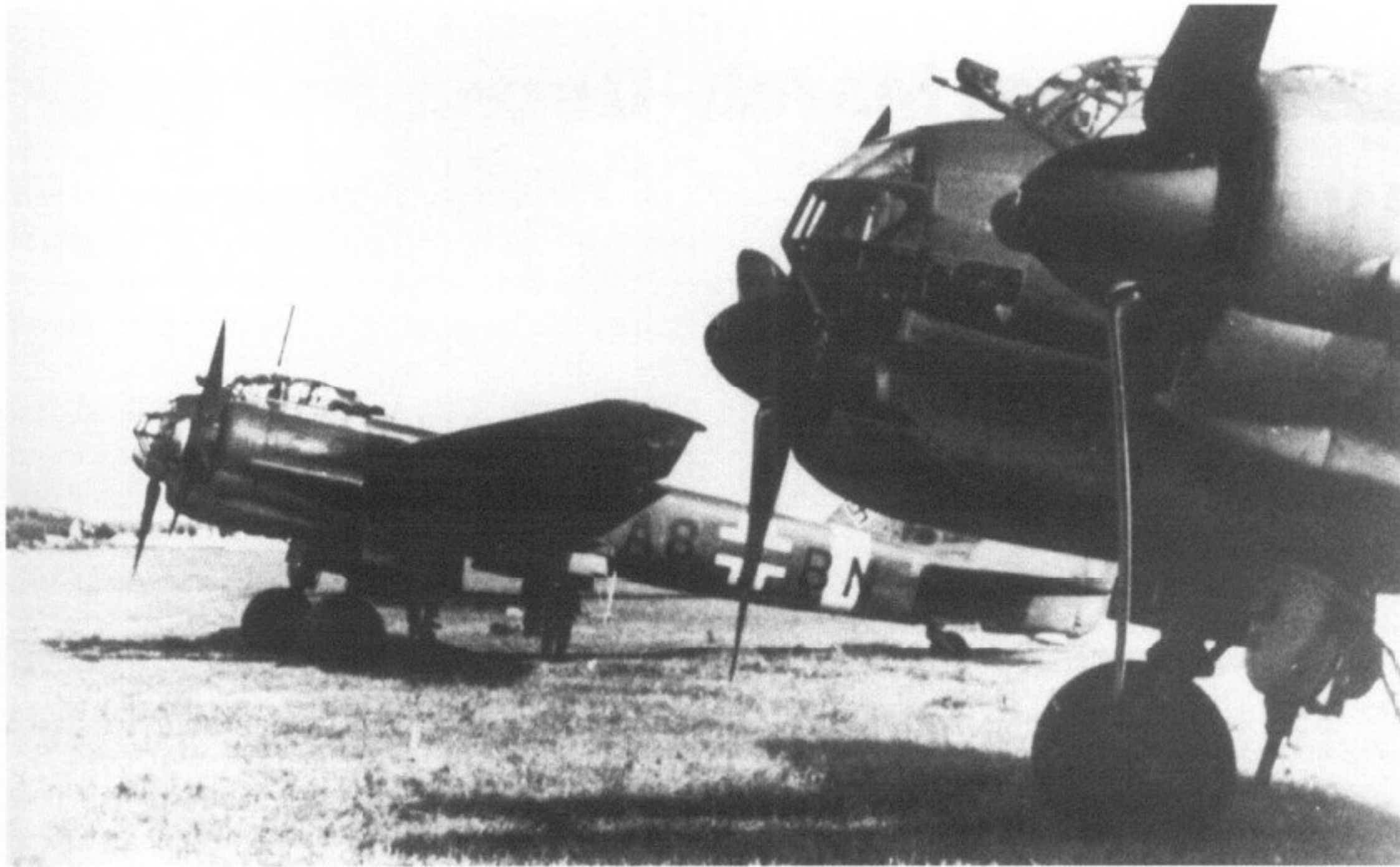
LEFT: A rare photograph of Ju 88 A-4s of 4./KG 102, probably taken at Grosseto 1942/43. Note the band around the fuselage of A8+BN. The large fitting in place of the more conventional gun sight on the forward firing 7.9 mm machine gun is a telescopic sight.
