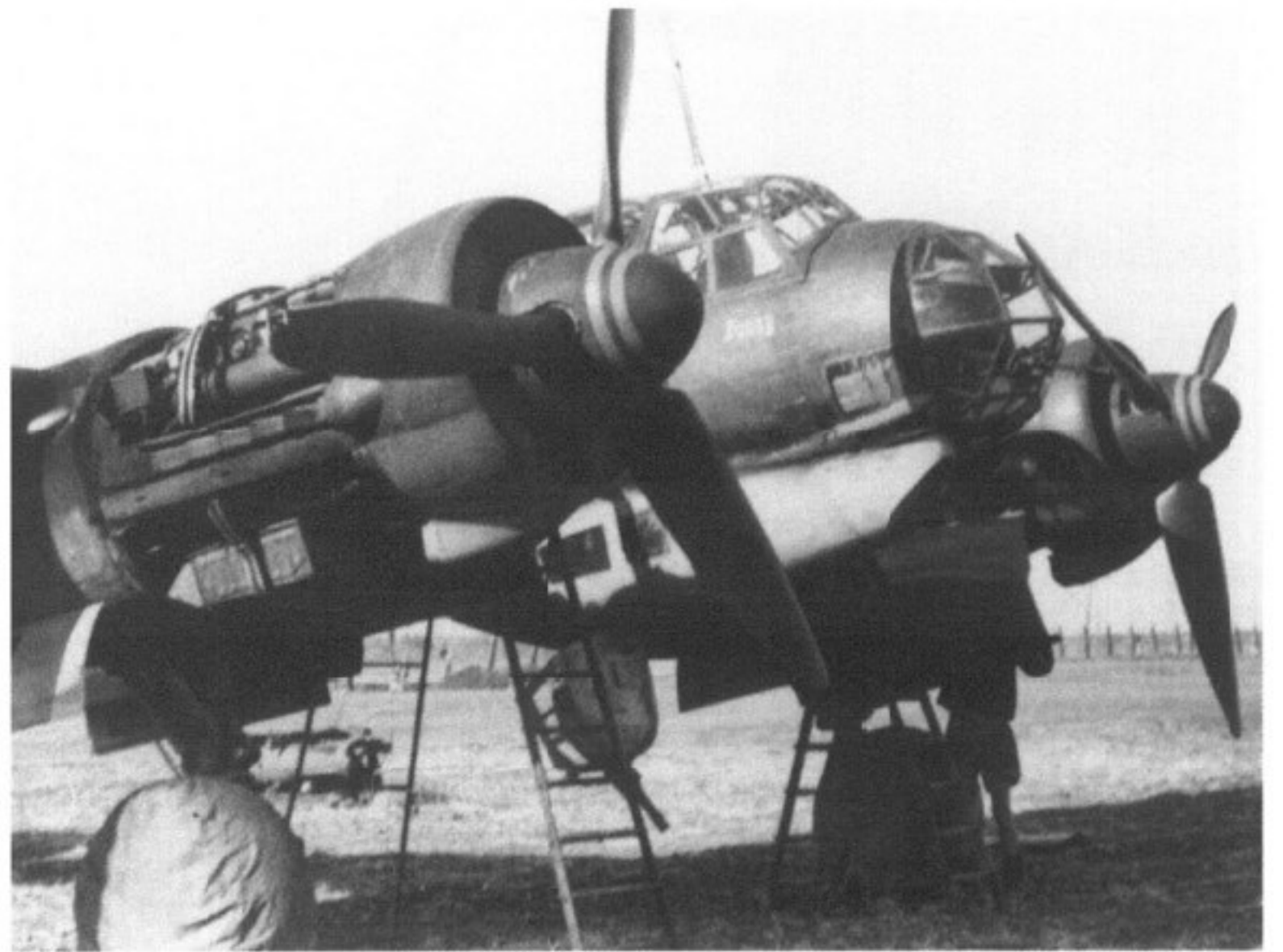
ABOVE: A Junkers Ju 88 of I./KG 77 at Gerbini, Italy in October 1942 receives some maintenance on its Jumo 211 V-12 engines from ground staff. Note the name 'Fanny' on the nose.
