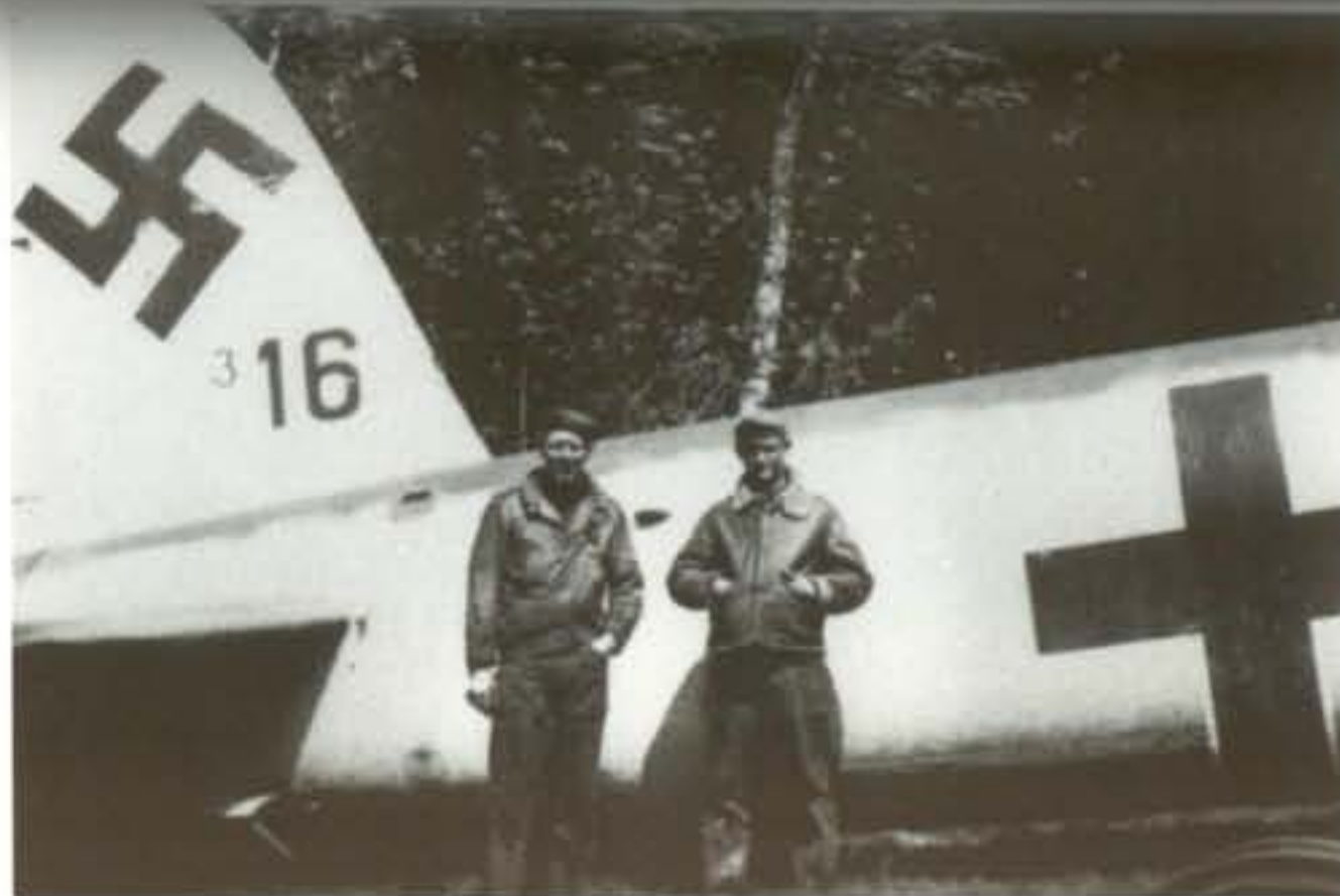
ABOVE: An Arado-built He 177 A-5 W.Nr. 550316 is seen here in an abandoned state after being found by US troops. Note how the last three digits of the Werknummer '316' are repeated on the tail fin and forward ventral gondola. The Heinkel also carries FuG 200 Hohentwiel ship search radar.
