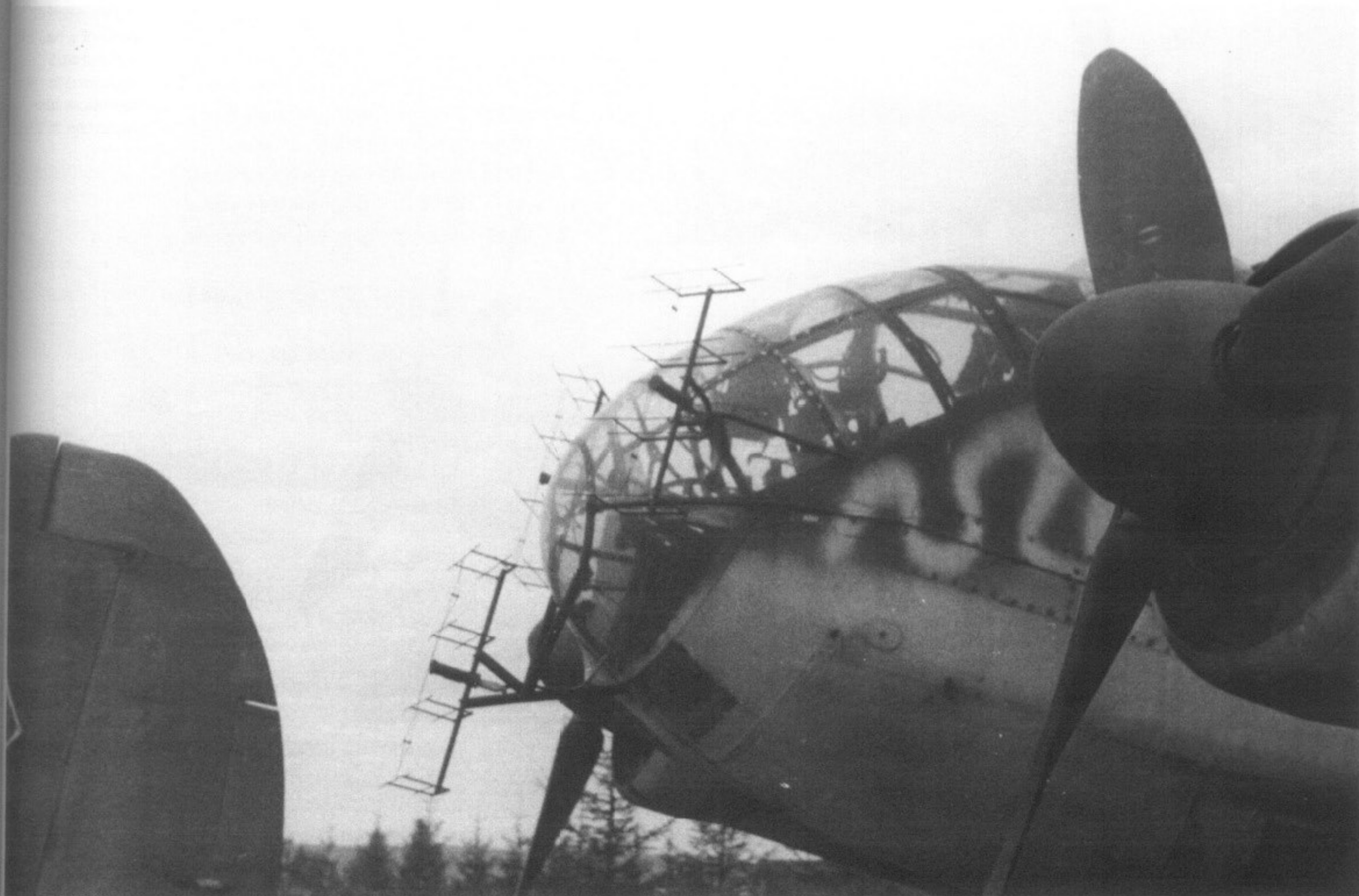
LEFT AND ABOVE: Ju 188s of KG 26 at Bardufoss. The aircraft above carries FuG 200 Hohentwiel ship search radar and the aircraft to the left carries the equipment for adjusting the steering of the torpedoes in flight, as evidenced by the dark bulge running down the starboard side below the cockpit.
