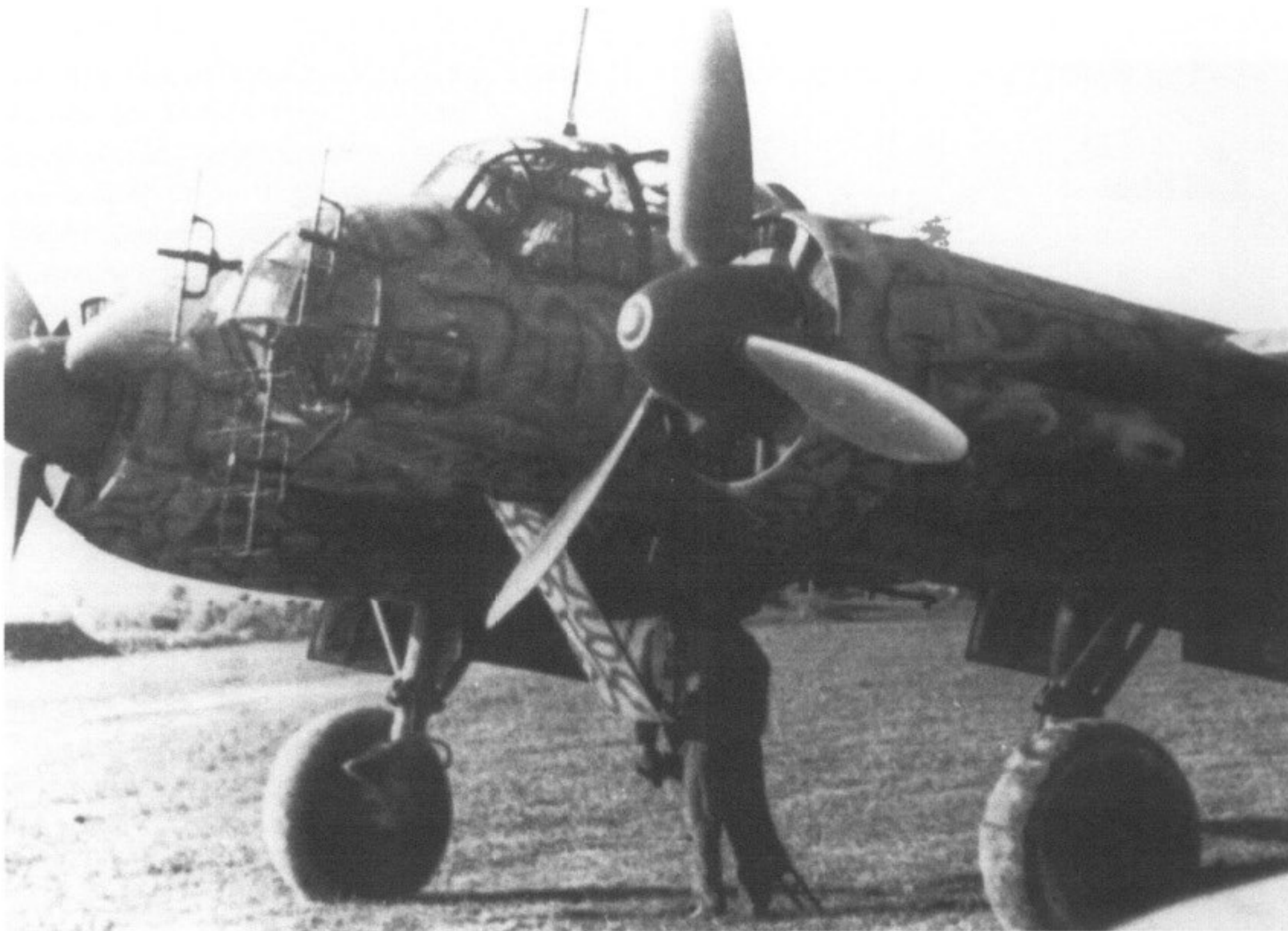
LEFT: Major Willi Solter's Ju 88 A-17 of I./KG 77 is seen here at La Jasse in the spring of 1944. Note the FuG 200 Hohentwiel ship search radar and the absence of the fuselage gondola, - sometimes found on this mark of Ju 88. The camouflage scheme is very non-standard and appears to be a mixture of RLM 79 sand-yellow oversprayed again in lines of RLM 76 and then again with further lines of either RLM 70 or 71 which was extended to the underside of the aircraft.
