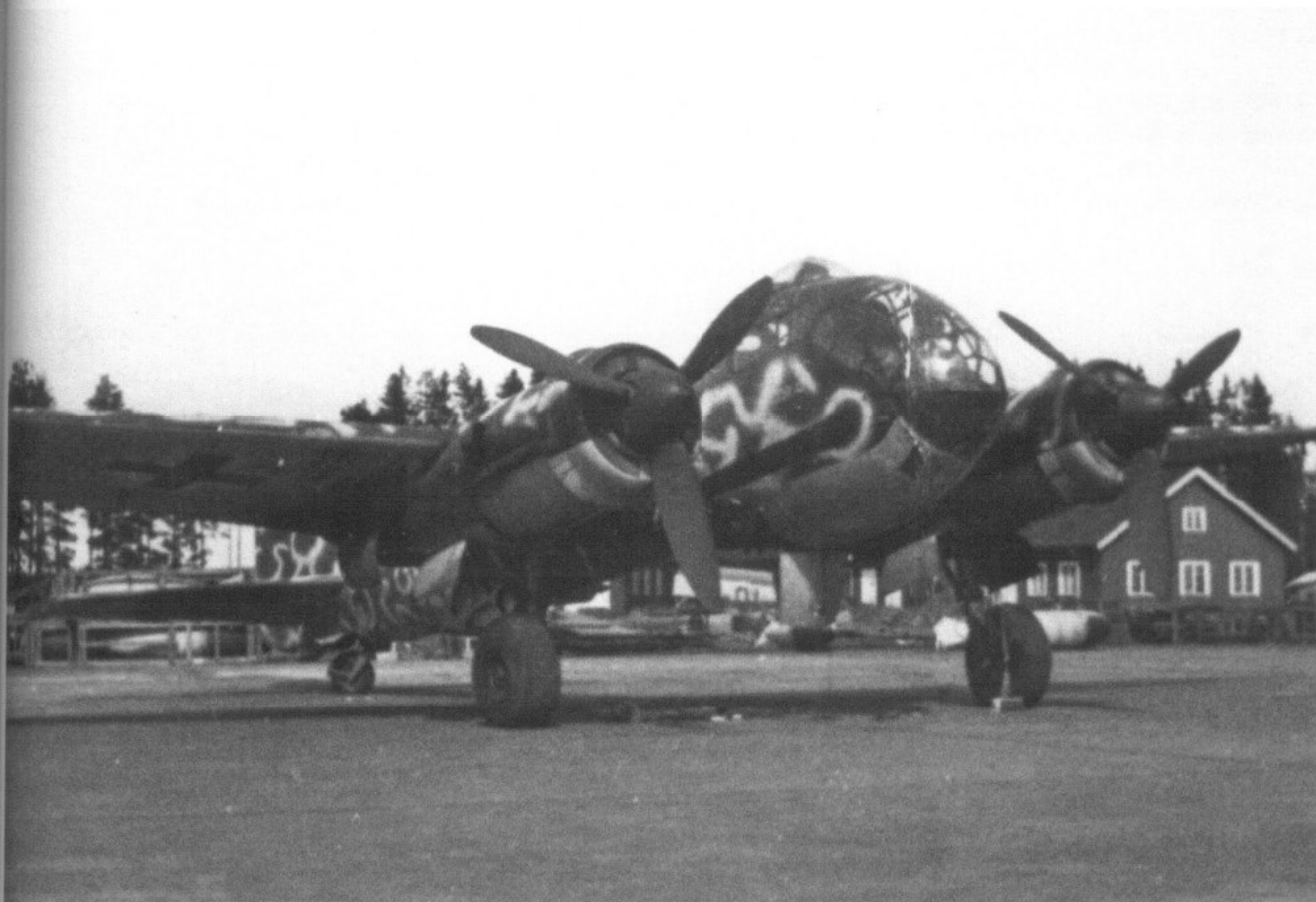
LEFT AND ABOVE: Ju 188s of KG 26 at Bardufoss. The aircraft above carries FuG 200 Hohentwiel ship search radar and the aircraft to the left carries the equipment for adjusting the steering of the torpedoes in flight, as evidenced by the dark bulge running down the starboard side below the cockpit.
