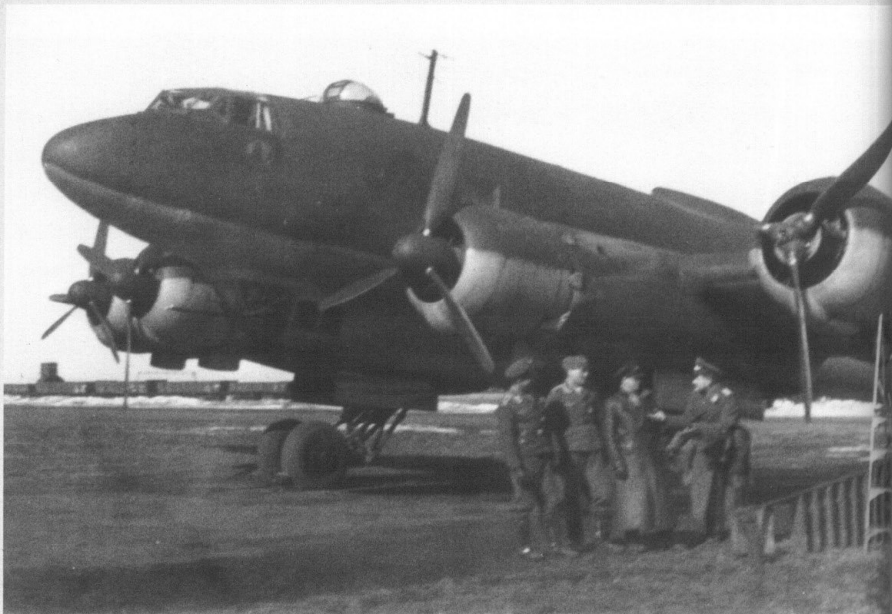
ABOVE AND RIGHT: Fw 200 C-3 W.Nr. 0074, coded F8+GH of 1./KG 40 seen at Aalborg, March 1941. The spinnerless port outer BMW-Bramo 323R-2 Fafnir nine-cylinder radial engine seems of interest to the two flight crew, one of whom is holding a hammer-like tool.
