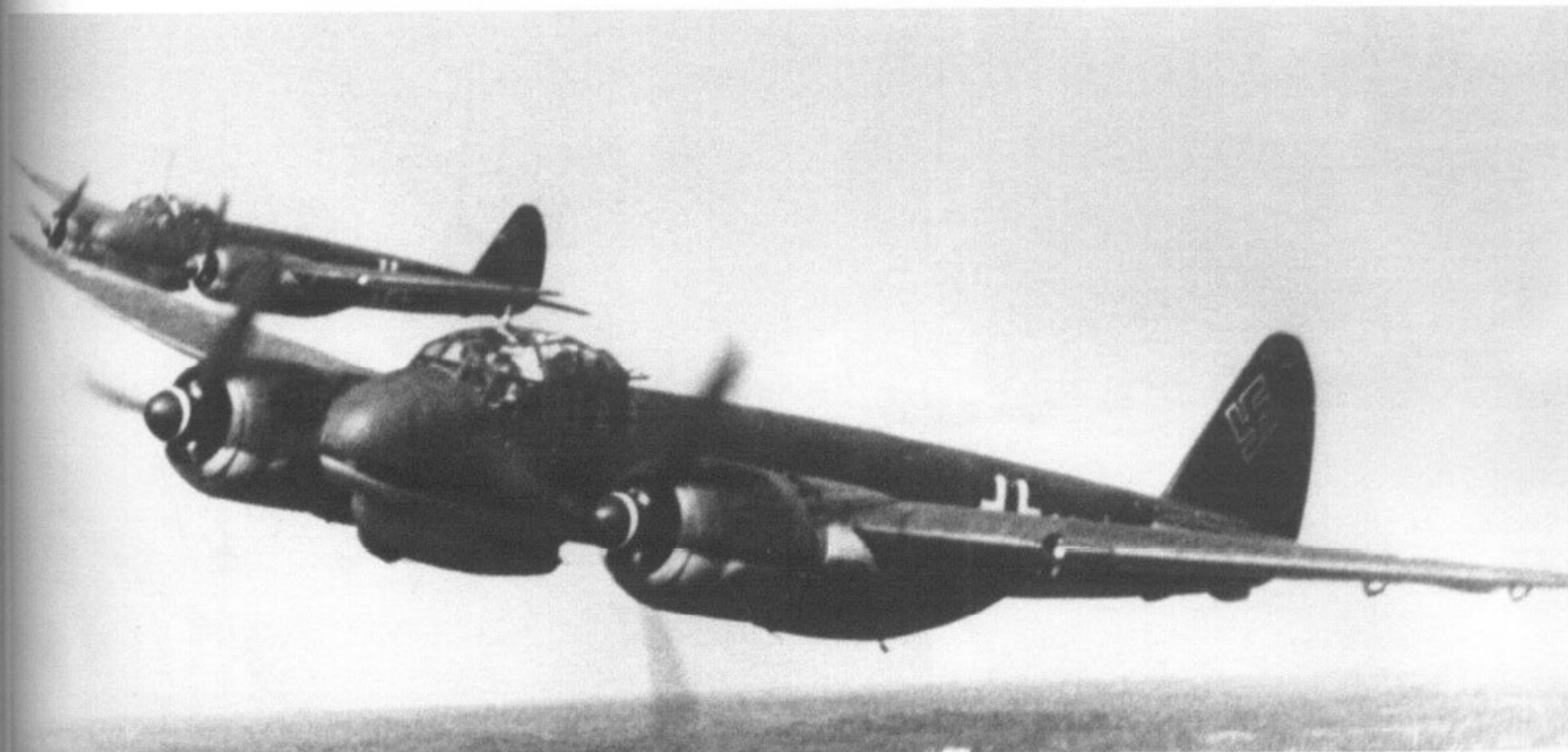
LEFT: Two BMW 801 MA powered Ju 88 R-2s of I./ZG 1. Although this variant was produced as a night fighter, the aircraft operated by ZG 1 were used in the role of high-speed destroyers. These machines were camouflaged in the splinter pattern of RLM 70/71 with RLM 65 underneath. The spinner tips were painted red with a white ring in the centre.
