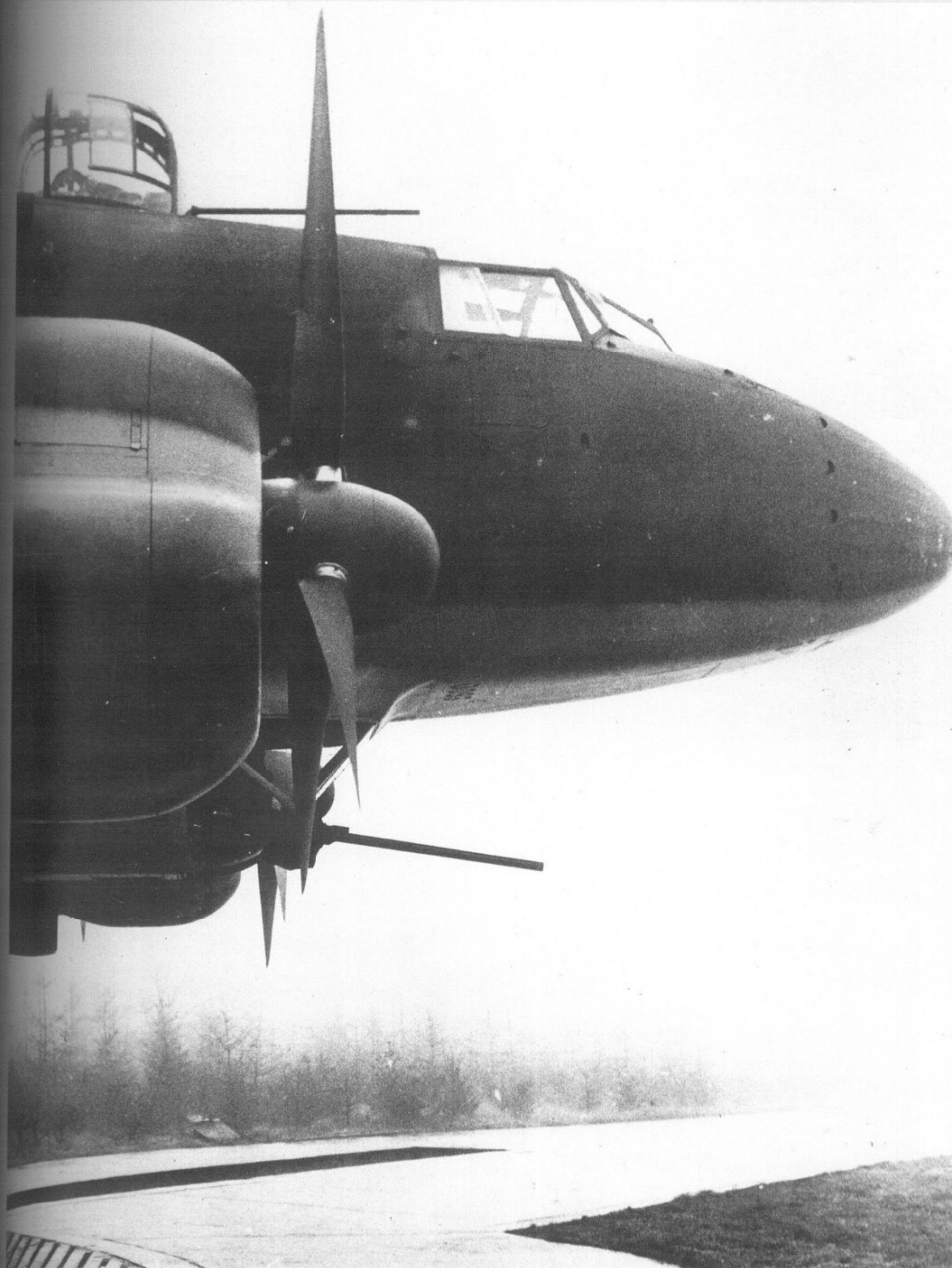
ABOVE: This Fw 200 C-3 or early C-4, features the improved armament introduced on these models - notably the forward dorsal hydraulically-operated HDL 151 turret housing a single 15 mm MG 151 cannon and another with a 300-round belt in the nose of the early style ventral gondola.
