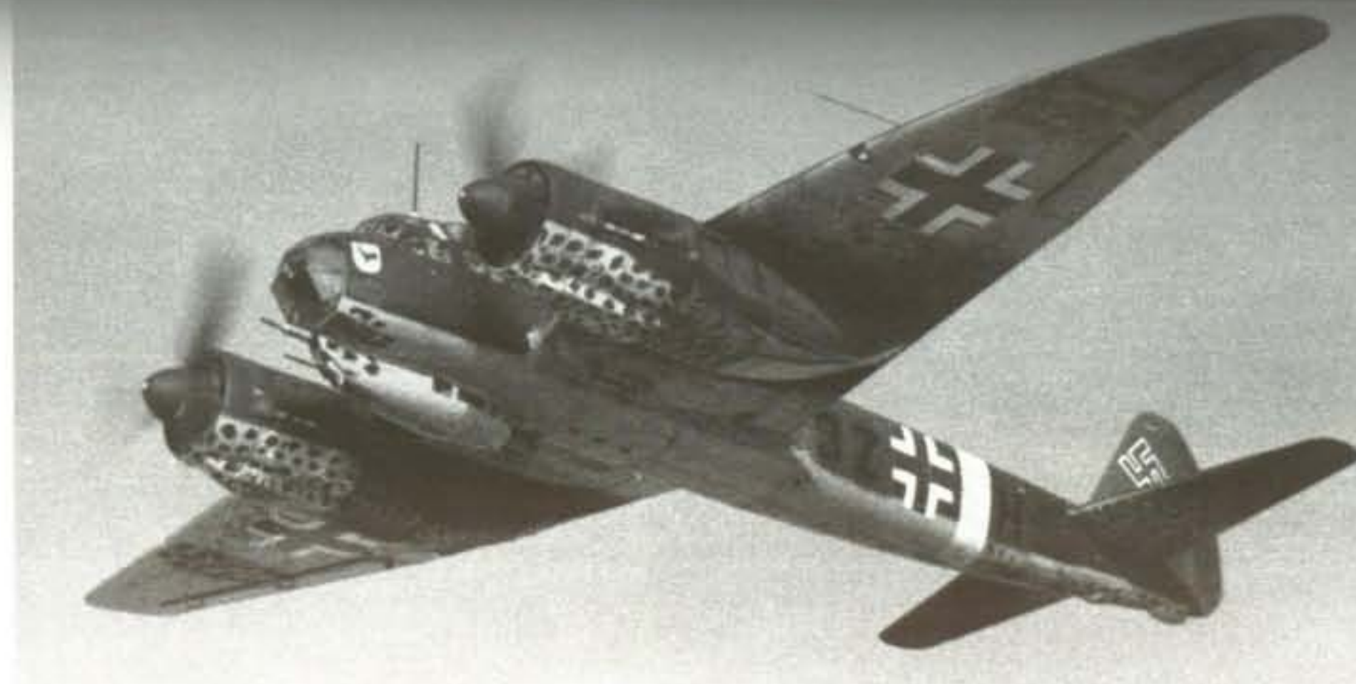
Left: A Ju 88 A-4 coded 3Z+EH of I./KG 77 with nose-mounted MG FF 20 mm cannon operating from Sicily late in 1942 on anti-shipping operations. The Lotfe bomb-sight has been removed from the nose of the ventral gondola to provide space for the cannon.
