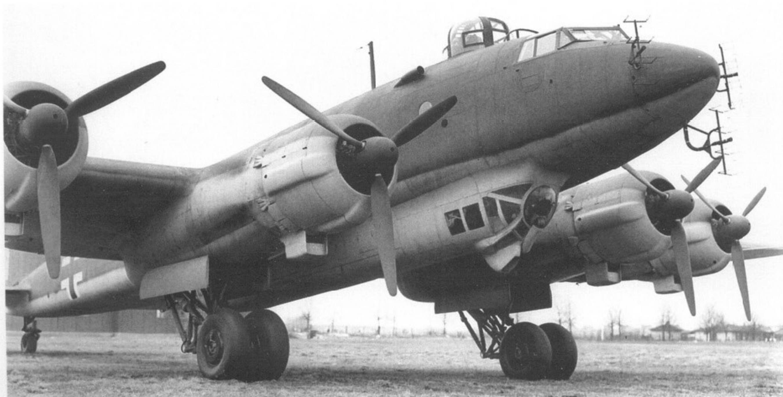
LEFT: A factory fresh Fw 200 C-4 Condor showing clear detail of many aspects of its structure and design. Note the installation of the FuG 200 Hohentwiel ship search radar, the Lotfe 7D bomb-sight and associated ventral glazing. The scoop on the upper fuselage is a cabin air inlet.
