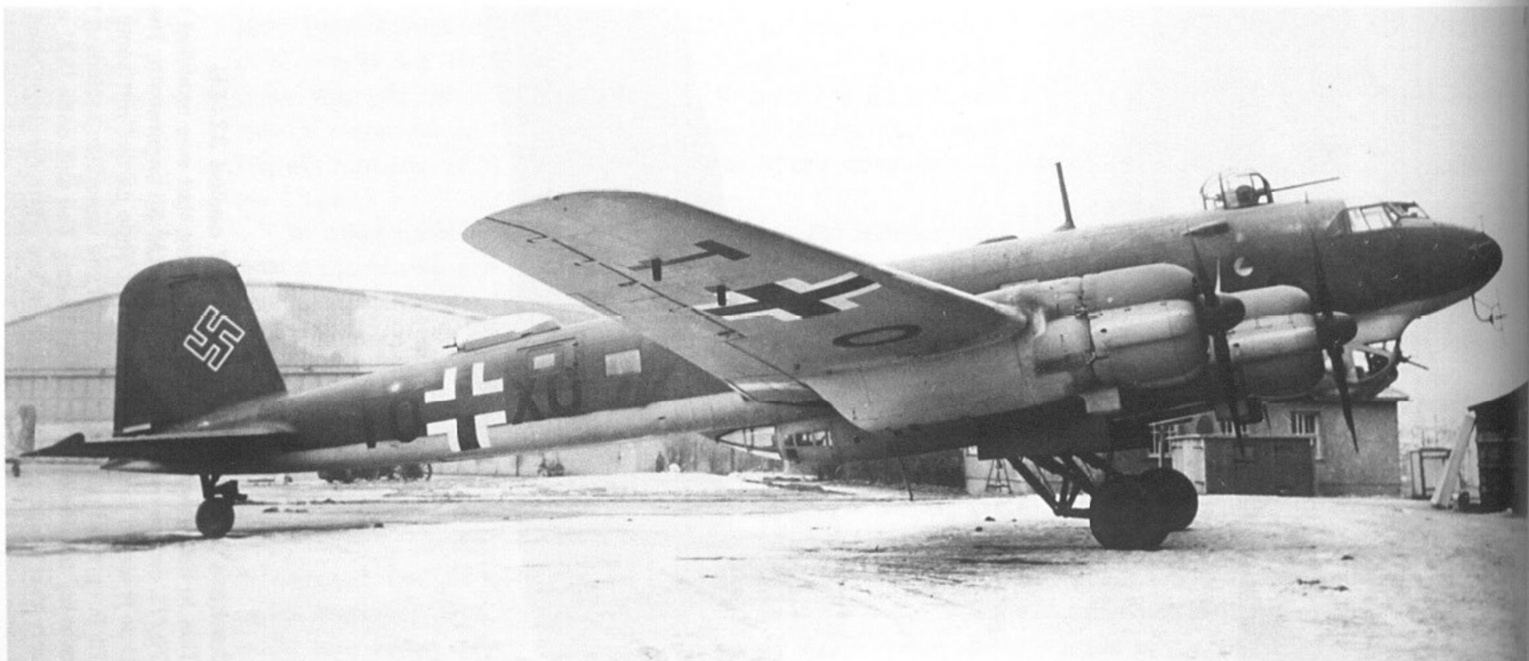
ABOVE: Fw 200 C-8/U10, W.Nr. 0259, factory coded TO+XO. The C-8 was the last production model and was intended specifically for the launching of Hs 293A missiles. Notable features of this aircraft are the deepened outboard engine nacelles (for carrying Hs 293s) and a forward, extended ventral gondola. Note the FuG 200 Hohentwiel ship search radar.
