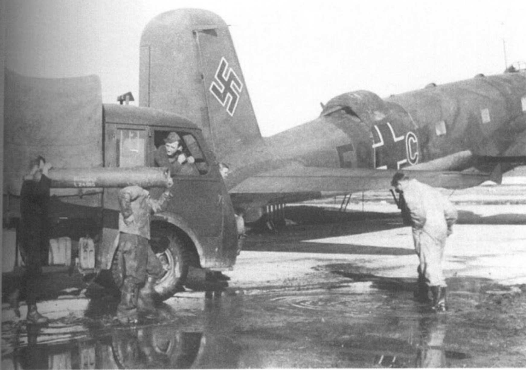
ABOVE: Two mechanics carry a cylinder, used to top up the on-board oxygen supply, towards a Fw 200 of 7./KG 40. This Condor carries the splinter pattern of RLM 72 and 73 with the code F8+CR in black with the aircraft letter 'C' edged in white. On many Fw 200s the fuselage Balkenkreuz had narrow white outlines.
