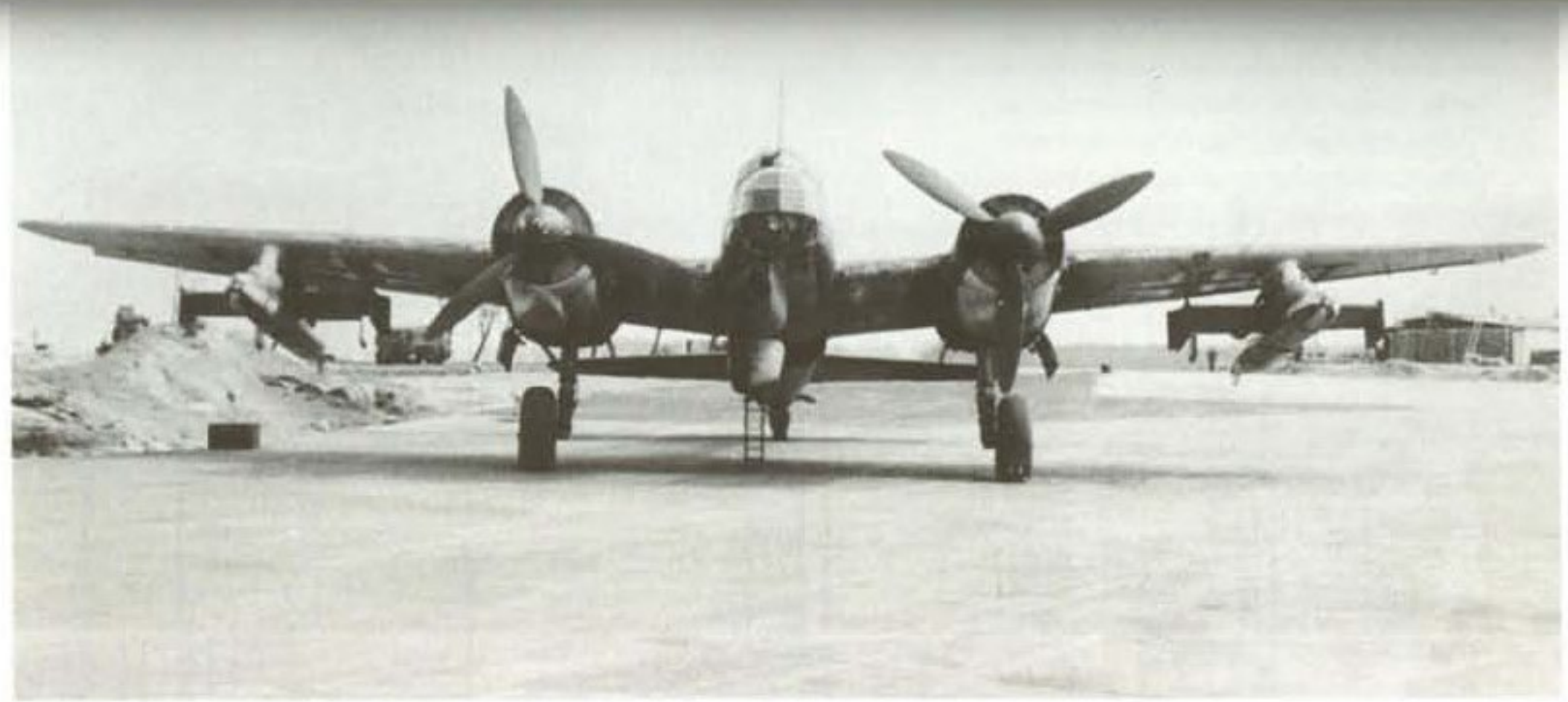
LEFT AND ABOVE: This Ju 88 A-4 was also used as a test aircraft for the L 10 mini-glider trials at the Gotenhafen-Hexengrund test centre. The two L10 torpedo carriers have been fitted with practice torpedoes, which were distinguished by the front warhead being replaced with a dummy head, which for testing purposes was painted in red and white segments.
